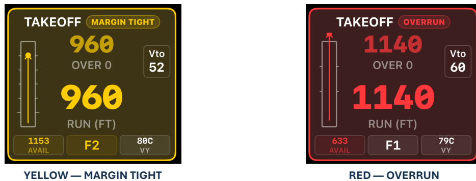
Figure 45. Takeoff cautions. Yellow means the applicable distance plus its required margin no longer fits; red means the predicted takeoff distance exceeds runway available.
