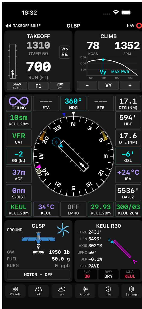
Figure 10. 2x2 HSI tile front. The center is the HSI instrument; the top and side rows are information chicklets, and the bottom row contains action chicklets.
