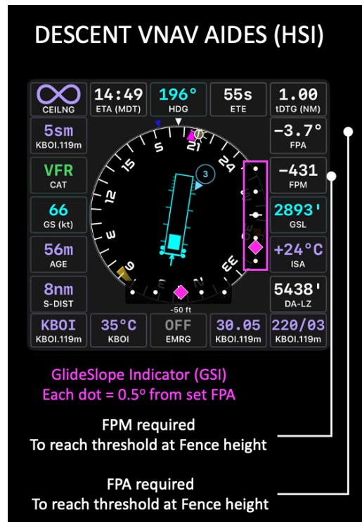
Figure 52. HSI descent vertical-navigation aids. The FPA and FPM chicklets show the profile required to reach the approach-end fence-height target. The GSI dots show deviation from the selected FPA; each dot represents 0.5 degree.
