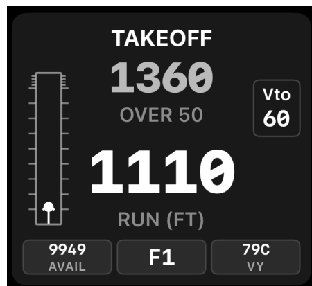
Figure 41. Takeoff tile with normal results. The upper value is distance over the selected fence height; the large lower value is the ground run to liftoff.
