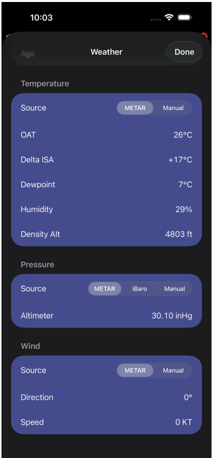
Figure 27. Weather source controls. Temperature and wind can use METAR or manual values; pressure can use METAR, iBaro, or a manual value.
